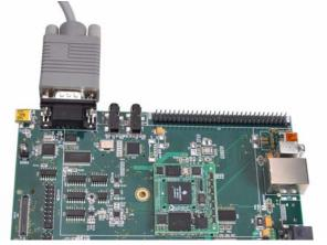
2. Connect the regulated 5V power supply to the appropriate power adapter for the region in which you are using the eXperimenter Kit.
