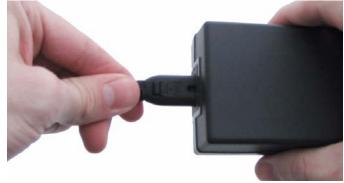
3. Plug the power adapter into an electrical outlet and the 5V line output connector into the power-in connector on the baseboard.
