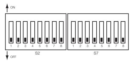
The S2 DIP switch is reserved for user application general purpose. The S7 DIP switch controls the processor's boot mode and several FET muxes on the baseboard. Table 2.10 describes the function of each switch.
