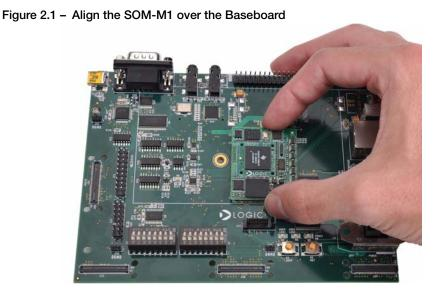
2. Press straight down on the SOM-M1, applying even pressure over the baseboard BTB socket connectors. See Figure 2.2.
